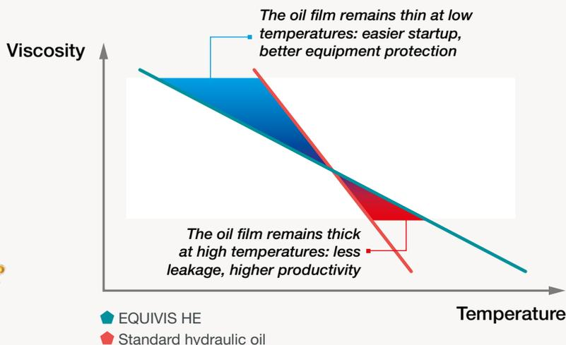
➤ **EQUIVIS HE maximizes performance in hydraulic operating systems**. Its thermal and mechanical stability helps to maintain ideal conditions for optimal operation.
